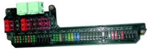
Front Power Distribution Box
